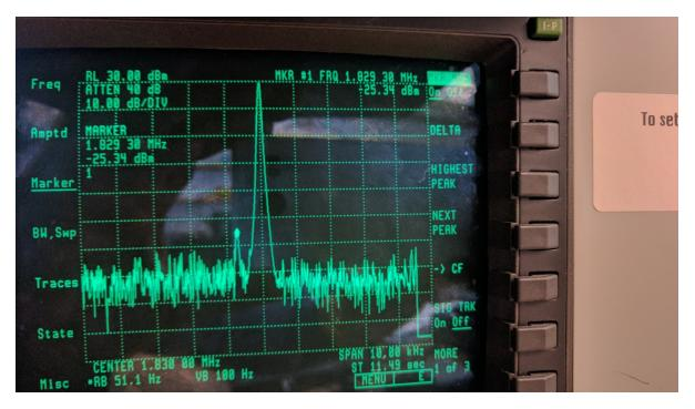
The spectrum analyzer noise floor, when the RXTX PTT is not keyed, is about -96 dB below the +30 dBm top scale, so all the noise shown in these photos is spurious sideband noise produced by the sound card.
