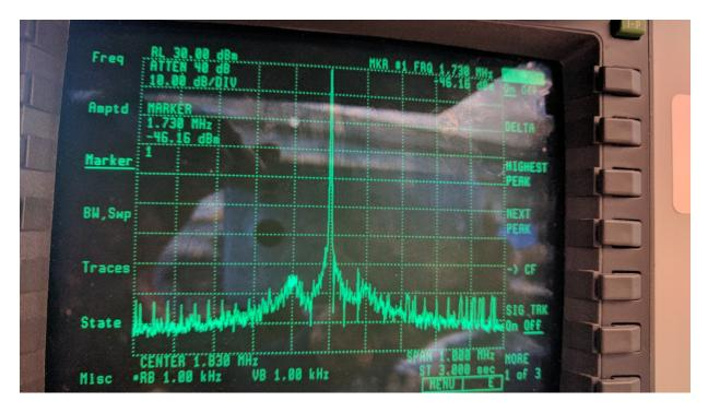
There is still significant noise close-in to the main signal, as shown in the next photo. This noise is about -70 dBc.
