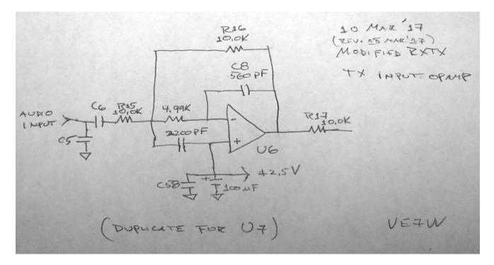
The effect of this filter is shown in the spectrum analyzer photos below. The RXTX is my modified version that covers the 2200, 630 and 160 mtr bands. As far as the sound card noise issue is concerned, the results should be the same for any band and for the standard RXTX. Power output is 1W, +30 dBm at 1.83 MHz, using PowerSDR in "tune" mode to generate a tone at 700 Hz above the LO.
